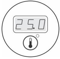
A digital display alternates between the actual water temperature and the set temperature. Simply press the integrated control button to select your ideal bathing temperature. An LED indicator shows the status of the heating function.
