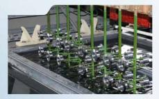
**Ultramodern electroplating facility**Corrosion protection through coating with bright nickel and nickel-chromium.
